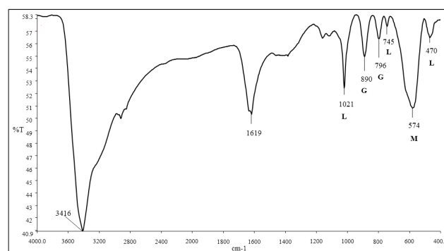
Fig. 2 FTIR spectrum of rust generated by salt spray (L = lepidocrocite, G = goethite, M = magnetite).
