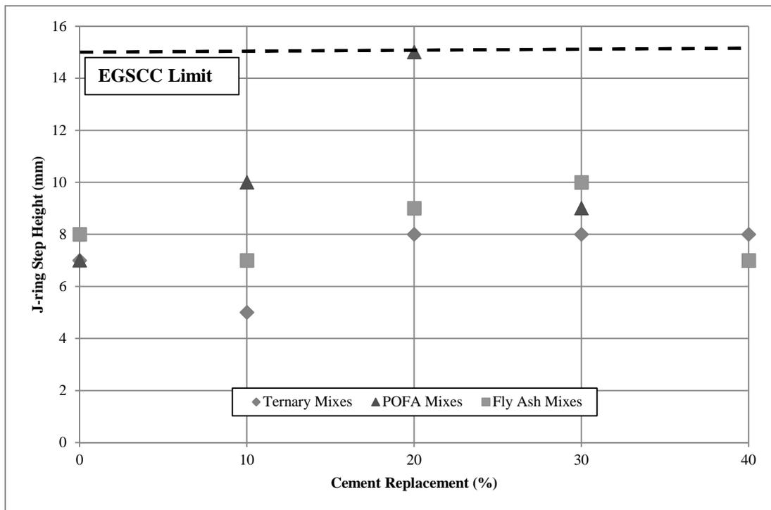
Fig. 10: Comparison of J-ring Step Height for Fly Ash, POFA and Ternary Blend.
