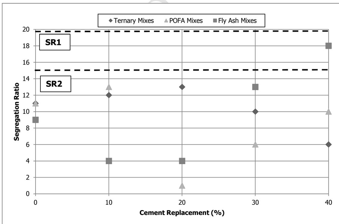
Fig. 11: Comparison of Segregation Ratio for Fly Ash, POFA and Ternary Blend.
