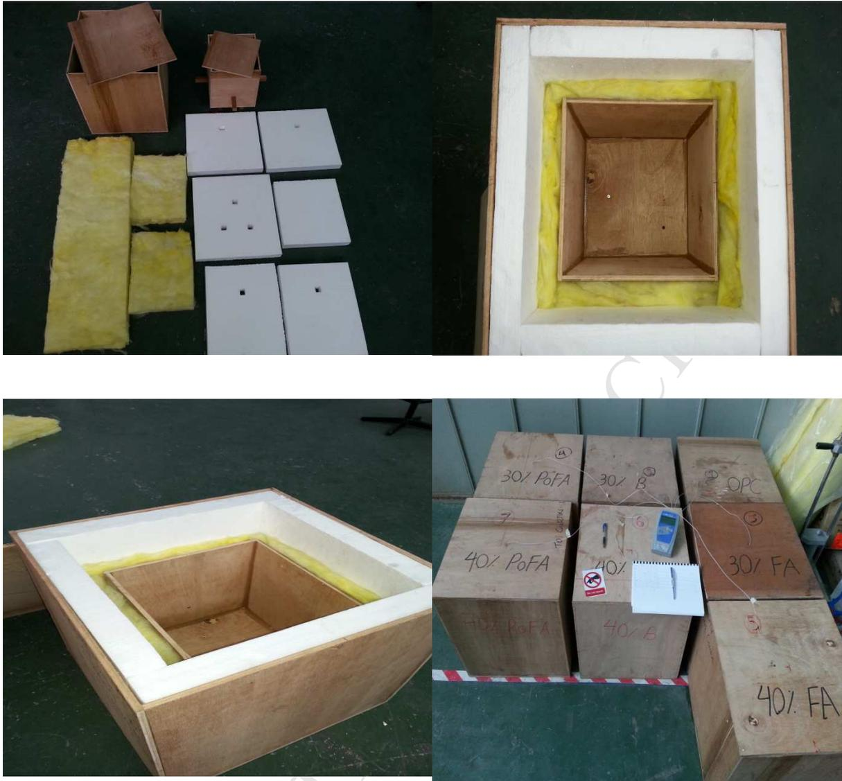
Fig. 5: Heat of hydration test set-up
