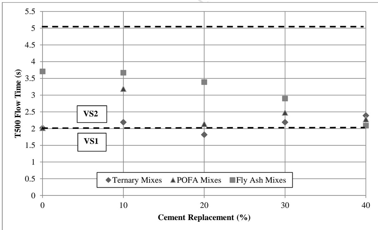
Fig. 7: Comparison of T<sub>500</sub> Flow Time for Fly Ash, POFA and Ternary Blend.
