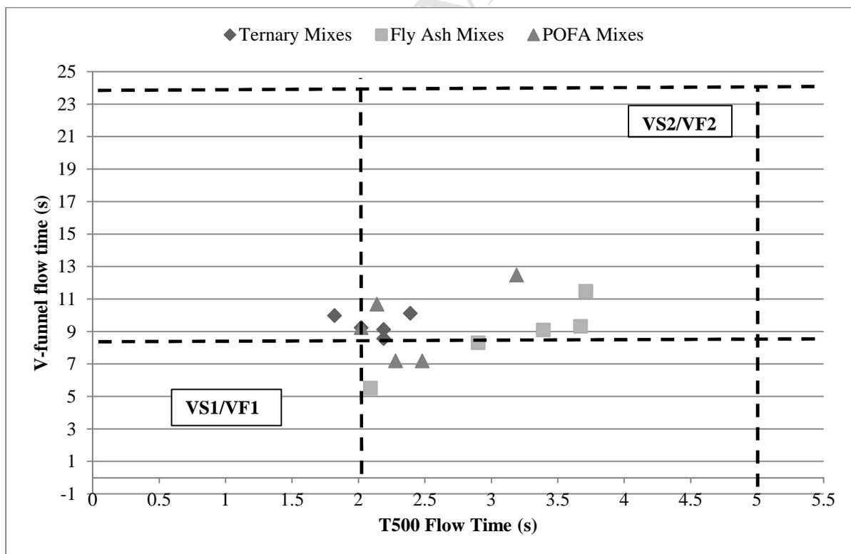
Fig. 9: Variation of viscosity classes with T500 and V-funnel flow times.
