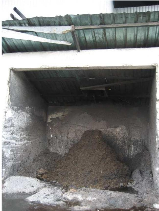
Fig. 4: POFA at the bottom of the furnace
