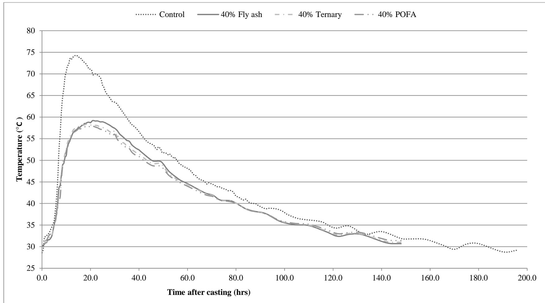
Fig. 14: Heat of hydration of Control and 40% blended concrete.
