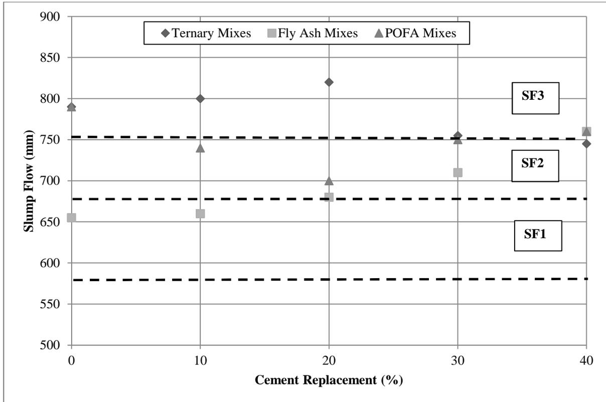
Fig. 6: Comparison of Slump Flow for Fly Ash, POFA and Ternary Blend.
