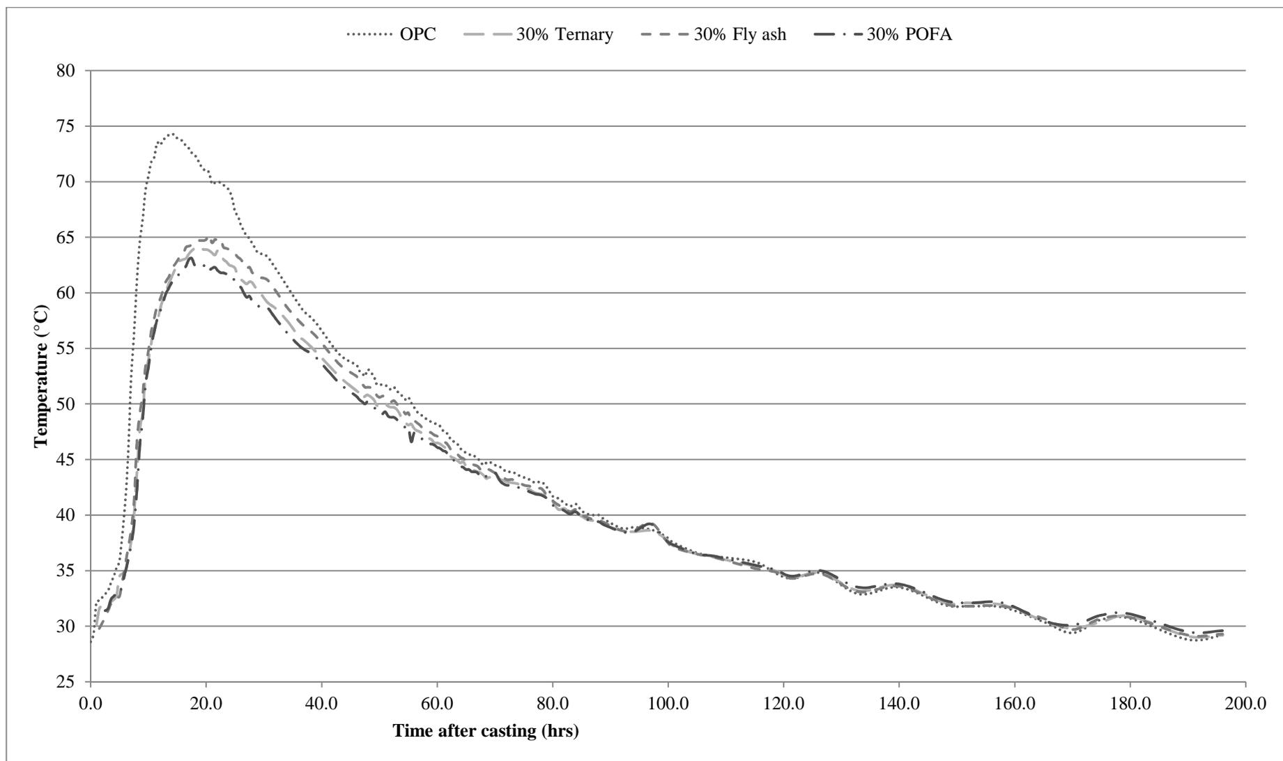
Fig. 13: Heat of hydration of Control and 30% blended concrete.
