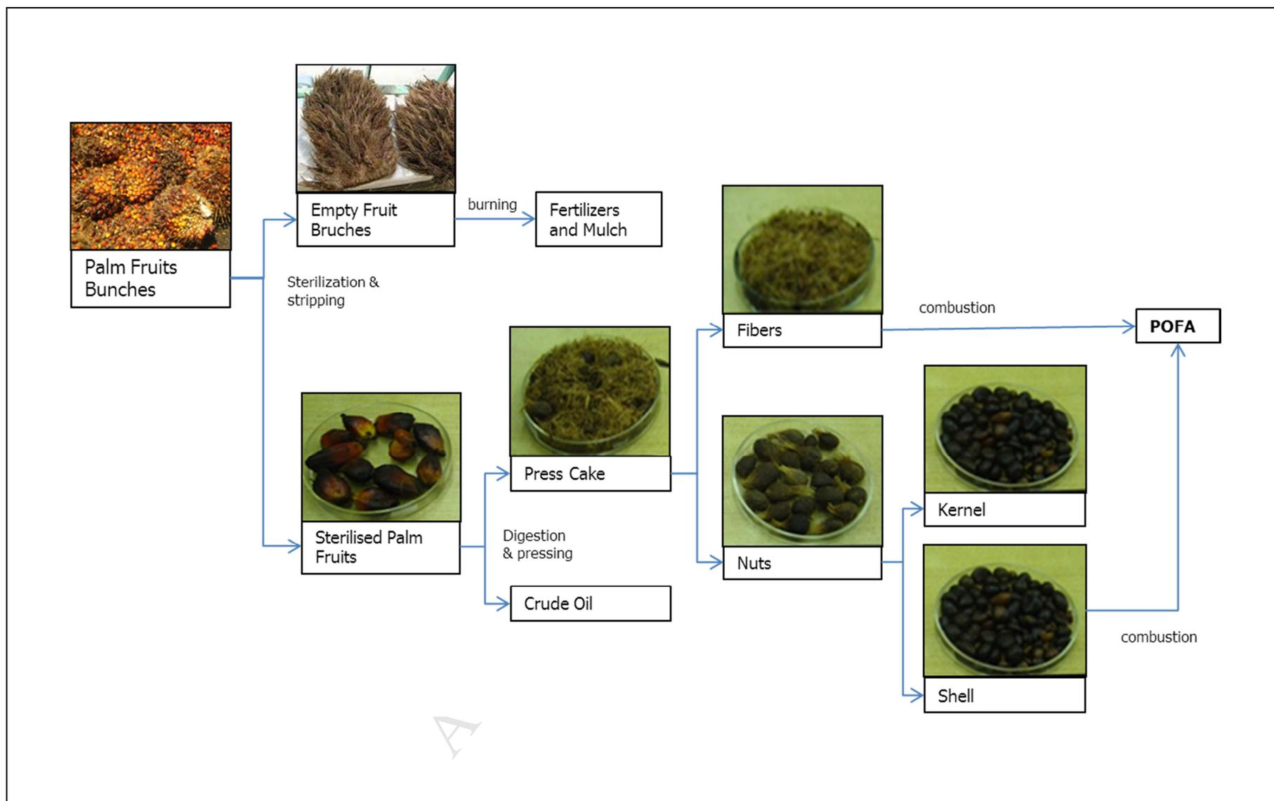
Fig. 1: The Schematic Diagram for Palm Oil Processing & POFA Production
