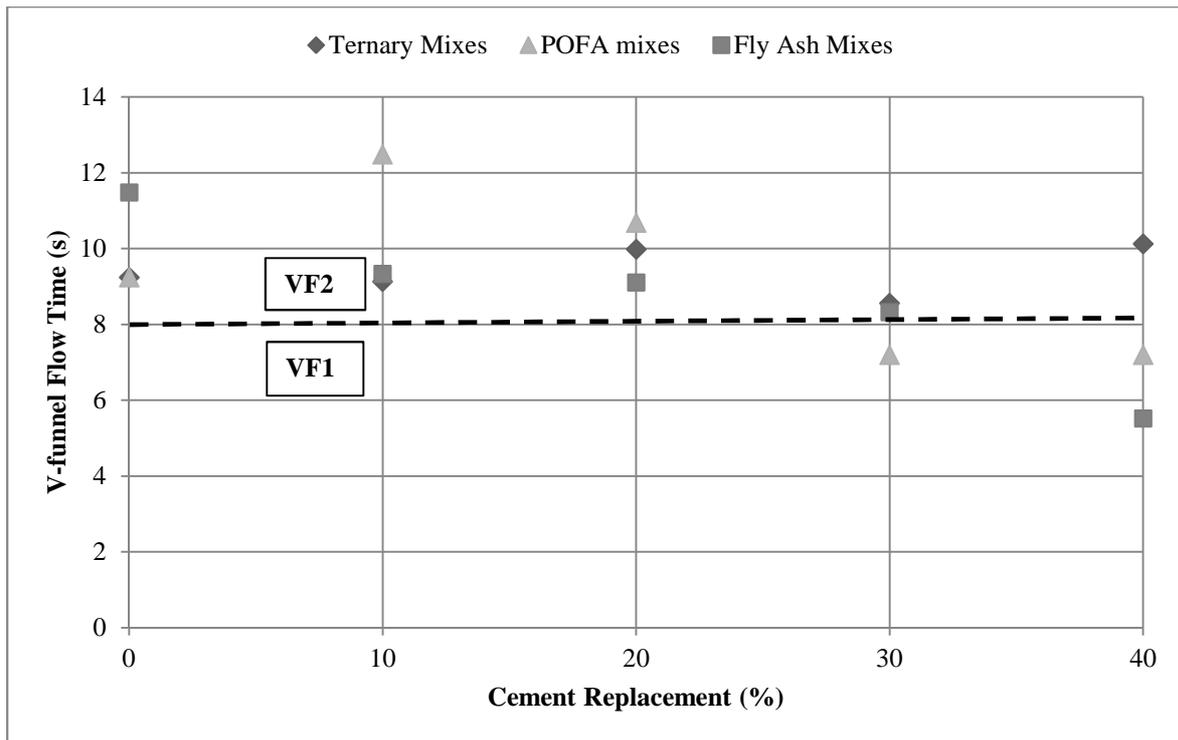
Fig. 8: Comparison of V-funnel Flow Time for Fly Ash, POFA and Ternary Blend.
