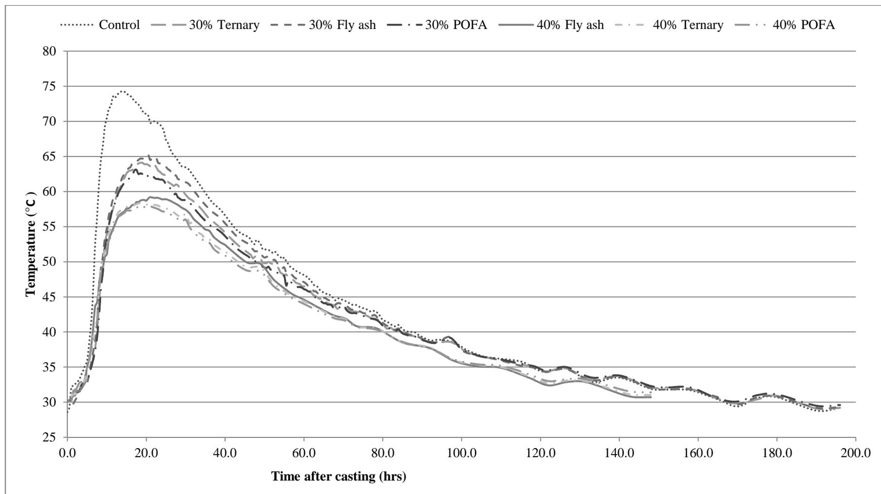
Fig. 12: Heat of hydration for all mixes
