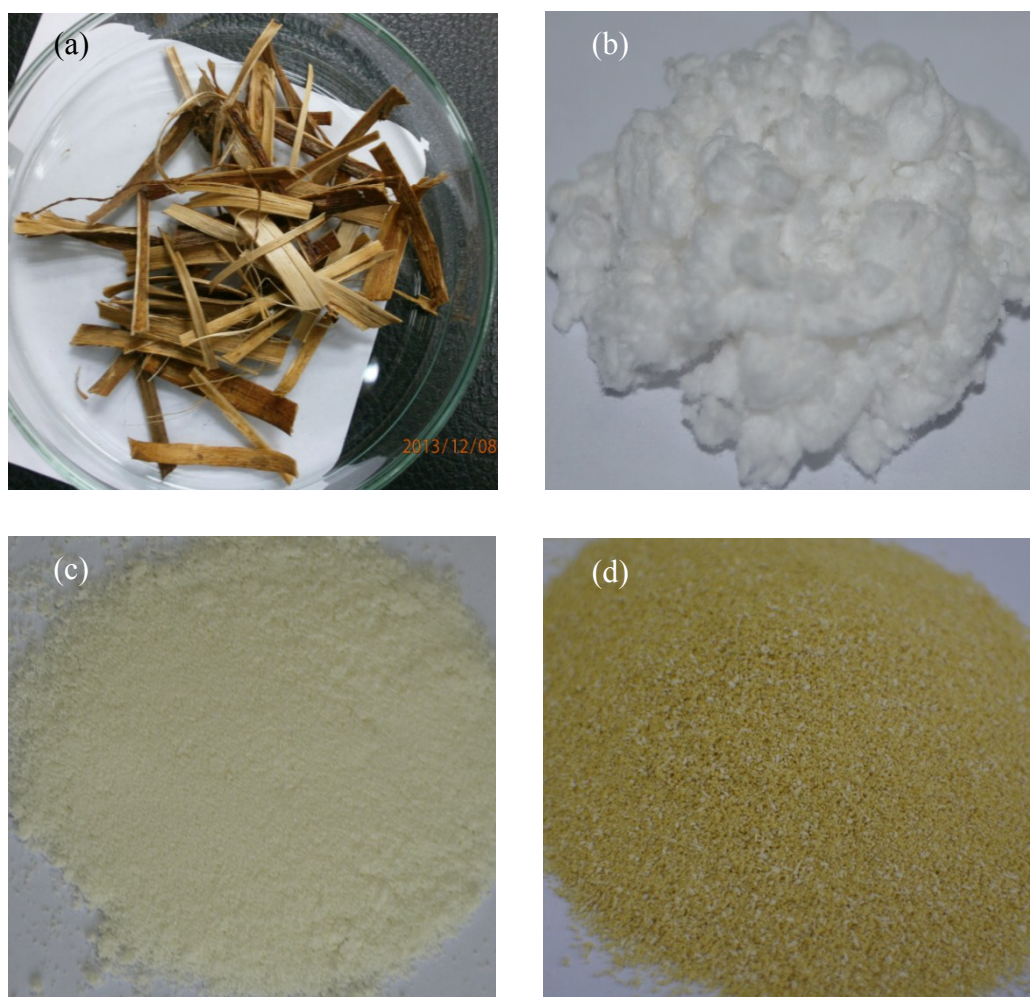
Fig. S1 Physical appearance of (a) kenaf bark, (b) kenaf cellulose, (c) poly(acrylonitrile) grafted kenaf cellulose and (d) poly(amidoxime) ligand.
