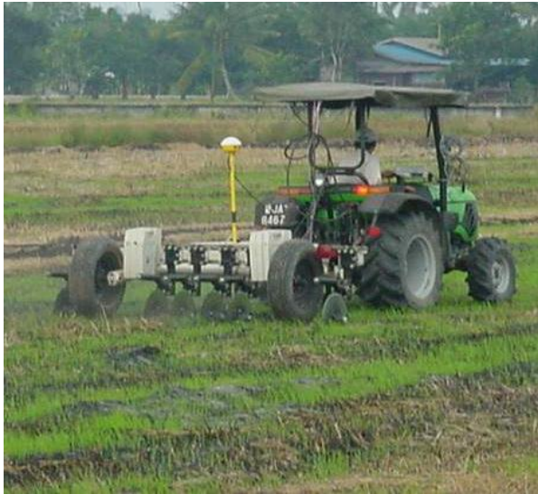
Figure 2 Soil ECa sensor integrated with Trimble Ag132 DGPS pulled by a tractor
