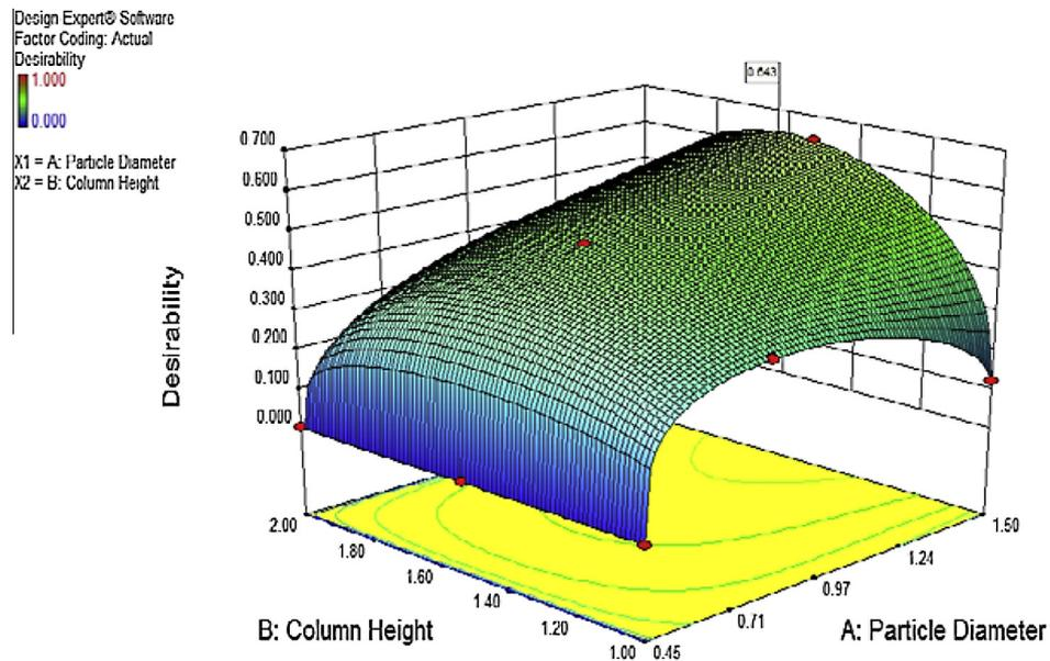
**Figure 4** Desirability graph of optimization done by using Design-Expert V8.0.7.1 program for determination of optimum value for particle diameter and column height.
