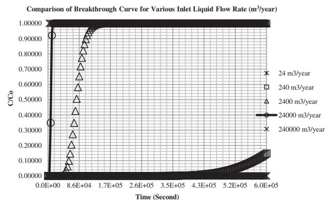
**Figure 6** Breakthrough curves for adsorption of phenol for various inlet liquid flow rates within 19.2 m height of activated carbon packed bed column with fixed initial phenol concentration of  $2.0189 \times 10^{-7}$  mol/l.
