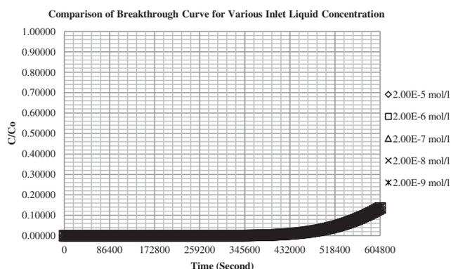
**Figure 7** Breakthrough curves for adsorption of phenol for various initial phenol concentrations within 19.2 m height of activated carbon packed bed column with fixed flow rate of 240 m<sup>3</sup>/year.
