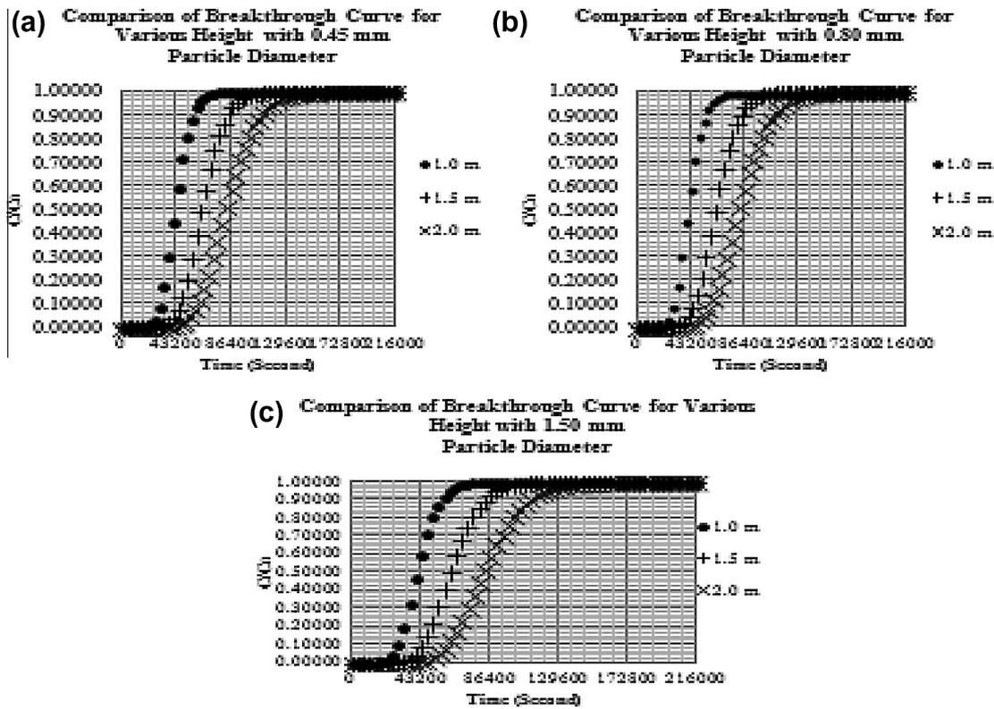
**Figure 3** Breakthrough curves for adsorption of phenol for various column heights of activated carbon filled with 0.45 (a), 0.80 mm (b), 1.50 mm (c) diameter of activated carbon particle.
