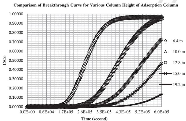
**Figure 5** Breakthrough curves for adsorption of phenol for various proposed column heights for real life application in water treatment plant.
