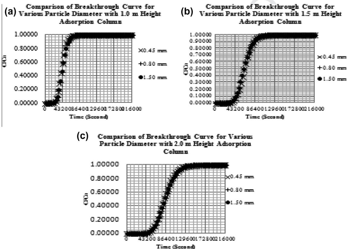
Q9 **Figure 2** Breakthrough curves for adsorption of phenol for various activated carbon particle diameters of activated carbon filled in 1.0 m (a), 1.5 m (b), 2.0 m (c) adsorption column.
