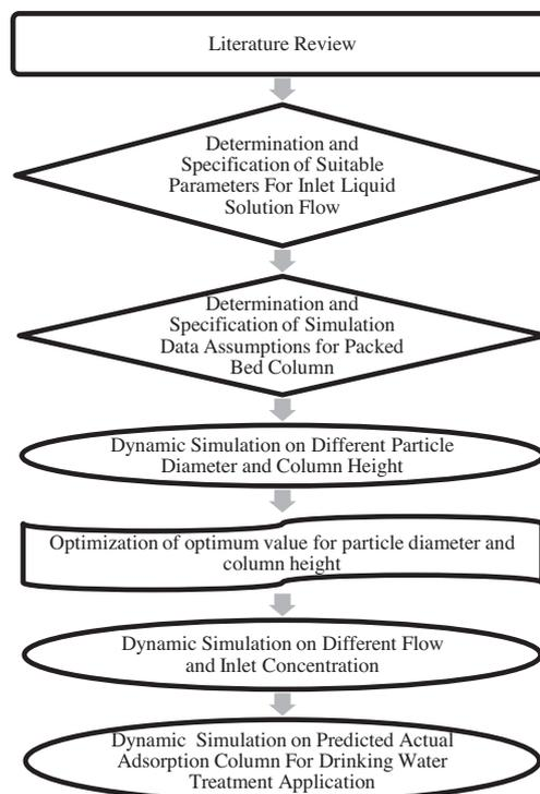
Figure 1 Chronology of dynamic simulation of phenol adsorption using aspen adsorption.
