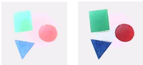
Fig.6. Image Acquired with Brightness, Contrast and Exposure of 0, 13, -5 (left) and -15, 20, -7(right) respectively
