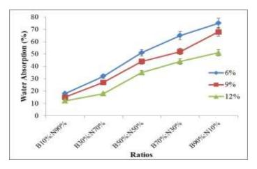
Figure 3. Percentage of water absorption of degradable bioplastic with 6%, 9% and 12% industrial cement.
