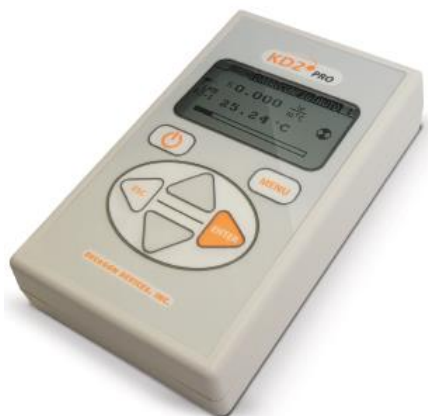
Figure 1 KD2 Pro thermal properties analyser controller [16]
