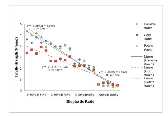
Figure 2. Trend graph for tensile strength of bioplastic sheets with different ratios of bioplastic and newspaper pulp fibres.
