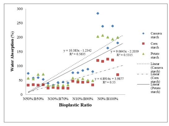
Figure 1. Trend graph for water absorption of bioplastic sheets with different ratios of bioplastic and newspaper pulp fibers.
