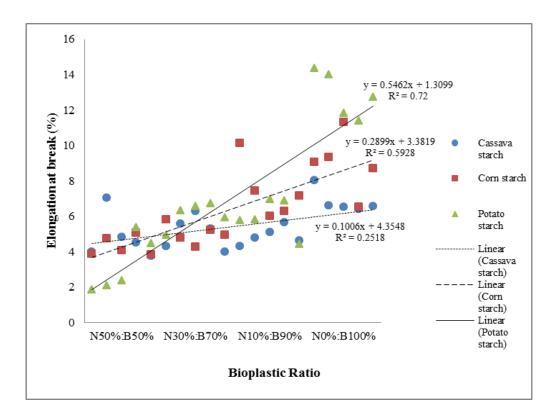
Figure 3. Trend graph for elongation at break of bioplastic sheets with different ratios of bioplastic and newspaper pulp fibres.
