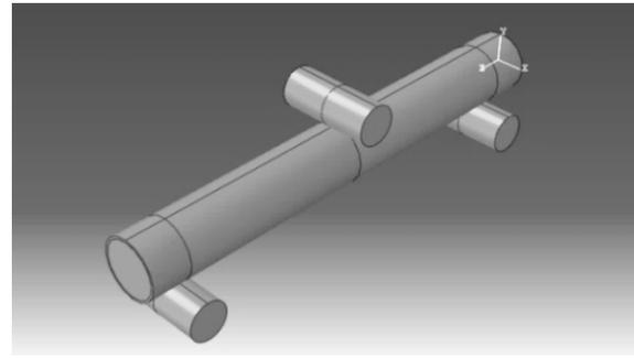
Fig. 2. Modelling three-point bending of polyurethane form-filled aluminium tubes in ABAQUS.
