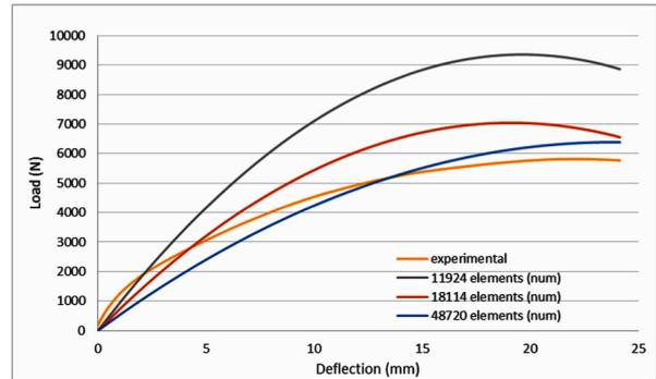
Fig. 12. Load-deflection of different mesh sizing and number of elements for foam-filled aluminium tubes (SL = 200 mm, D/t = 26.7) by 3-point bend loading.
