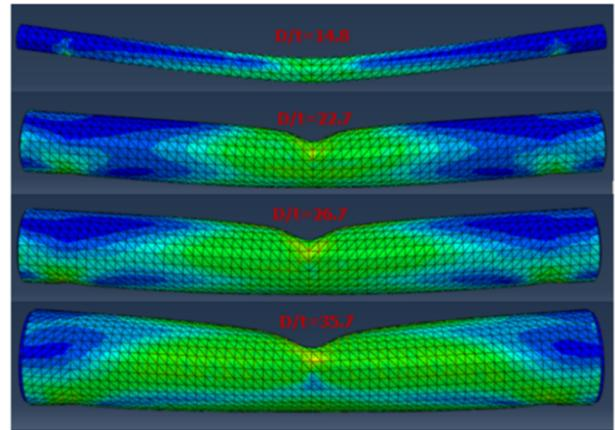
Fig. 8. Deformation model of filled-tubes with varying D/t ratios and fixed span length of 250 mm.
