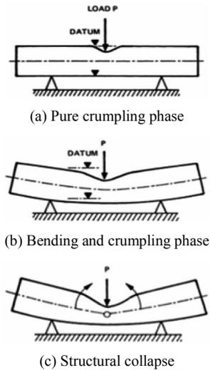
Fig. 1. Modes of deformation of tubular under transverse load [3].
