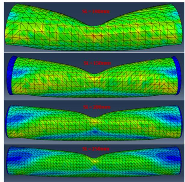
Fig. 9. Deformation model of filled-tubes with varying span lengths and fixed D/t ratio of 35.7.
