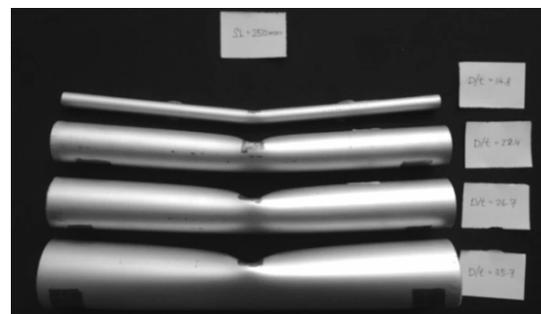
Fig. 5. Deformed PU-filled aluminium tubes of varying D/t ratio with fixed span length of 250 mm.
