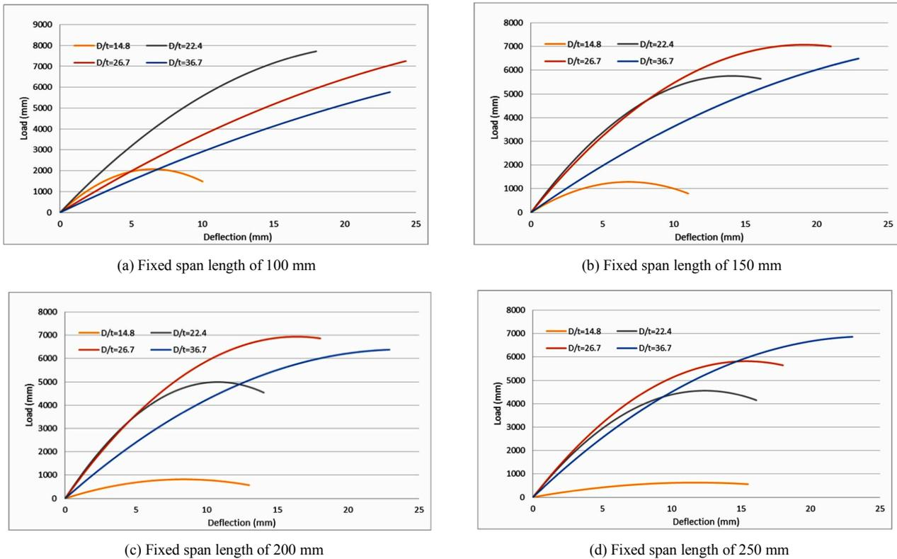
Fig. 6. Load-deflection curves for foam-filled tubes of different  $D/t$  ratios with fixed span lengths.
