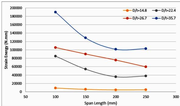
Fig. 11. Numerical strain energy vs span length for various D/t ratios of foam-filled Al-tubes by 3-point bend loading.
