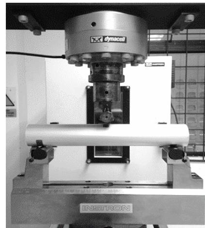
Fig. 4. PU-filled aluminium tube subjected to three-point bend loading on INSTRON machine.
