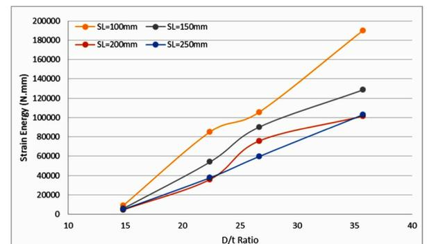
Fig. 10. Numerical strain energy vs D/t ratio for various span lengths of foam-filled Al-tubes by three-point bend loading.
