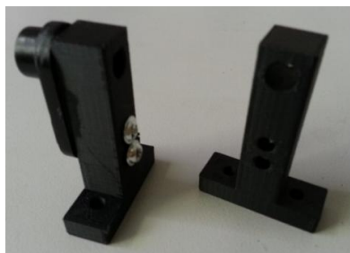
(b) Printed robot legs
