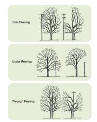
Fig. 1: Pruning method being used by Nasional Grid
