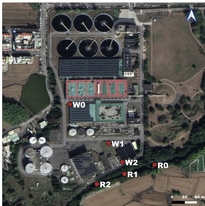
Fig. 1. Sampling locations in Taichung. W0 (influent), W1 (primary and secondary treated wastewater), and W2 (chlorinated effluent) were located in the wastewater treatment plant. R0, R1, and R2 were in the river that receives the effluent at 50 m upstream of the effluent outlet, the outlet, and 50 m downstream of the outlet, respectively.
