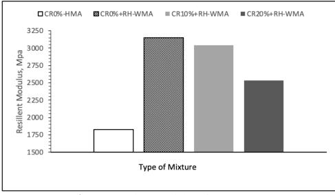
Figure 2. Resilient modulus of CR mixtures
