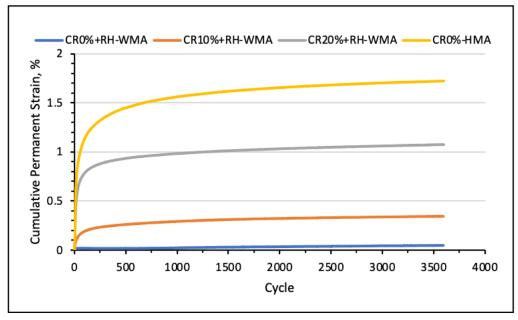
Figure 3. Effects of CR addition on cumulative permanent strain
