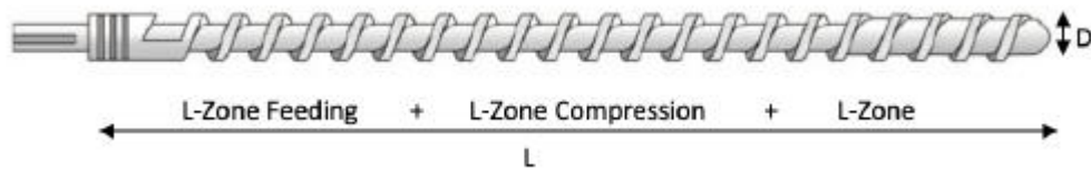
Figure 2.2: Extrusion Screw Zone
