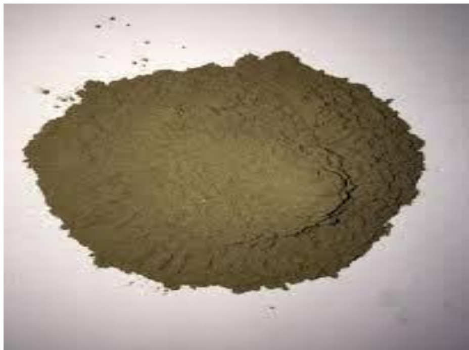
Figure 2.2 : Eco Process Pozzolan Ash Source : Yunus, E. et al. , (2020)
