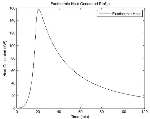
Figure 5. Exothermic heat profile under nominal case
