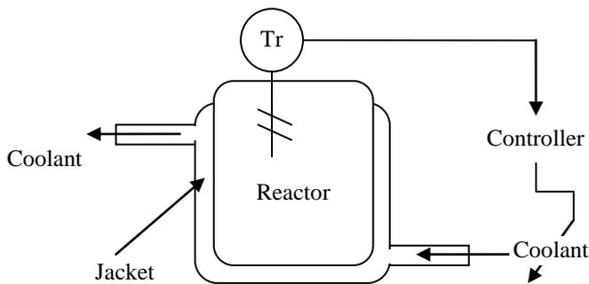
Figure 1. Batch reactor diagram
