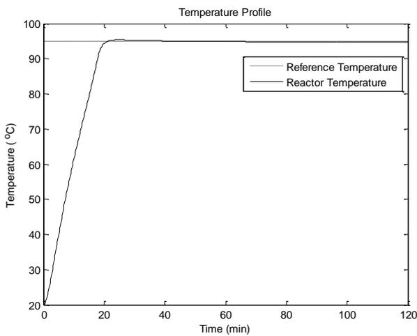
Figure 4. Performance of PID controller at nominal case
