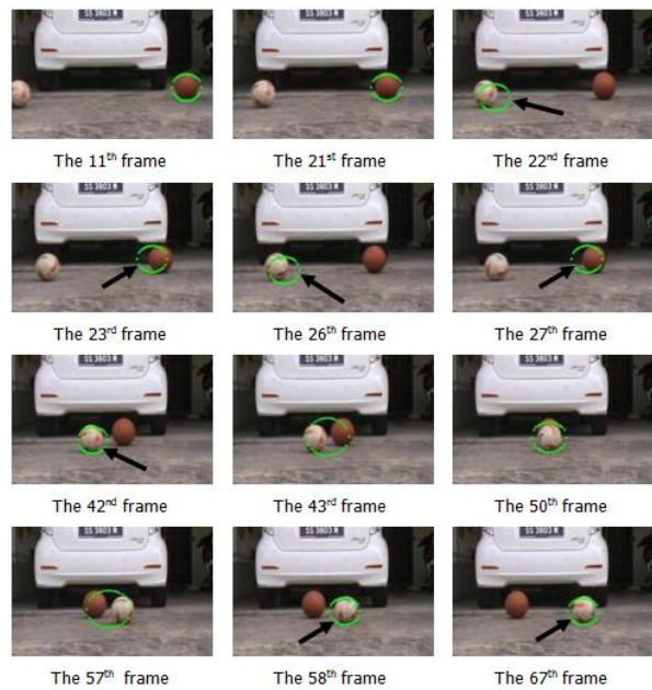
Figure 5. The experimental result of occlusion of two moving objects (KF)
