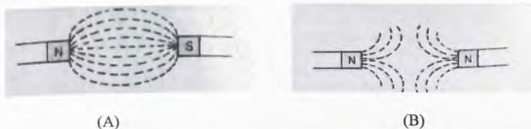
Figure 2.7 (A) Two unlike poles. (B) Two like poles
