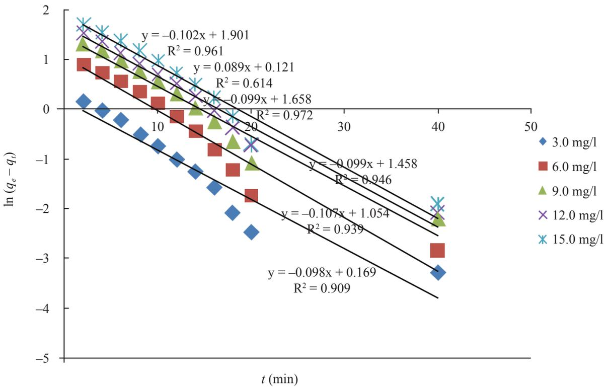
Figure 8. The pseudo-first-order kinetic model for MB dye adsorption onto rambutan skin biosorbent.
