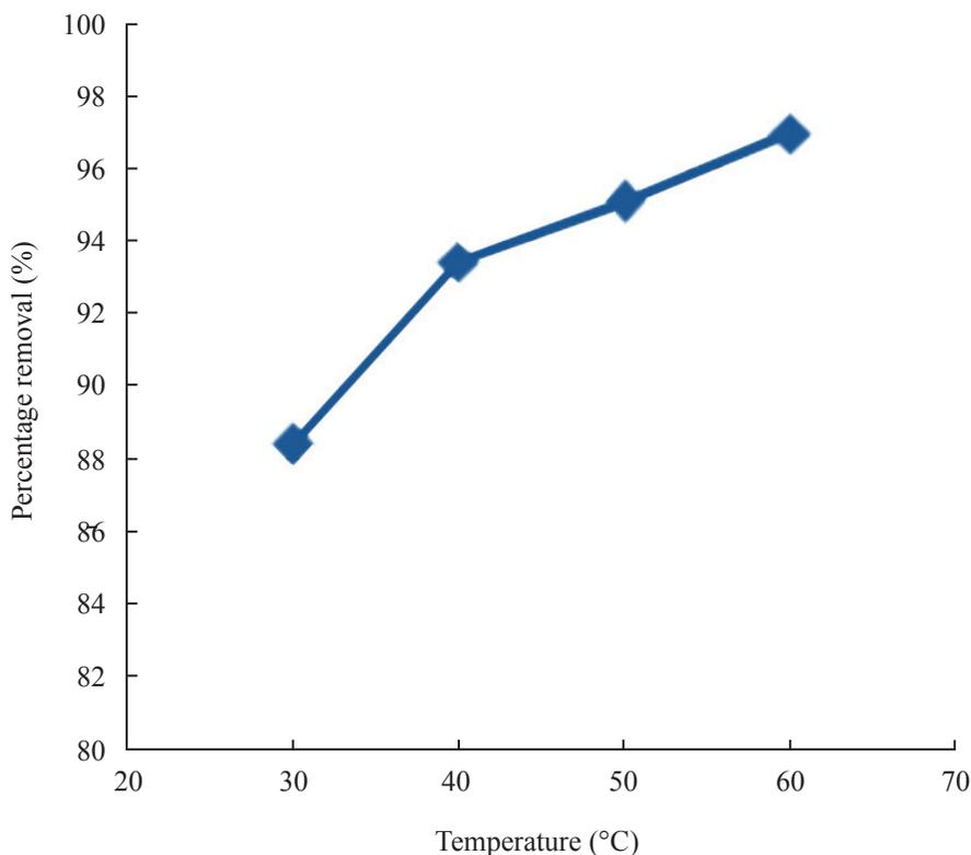
**Figure 3.** The effects of the solution temperature on MB dye adsorption percentage.
