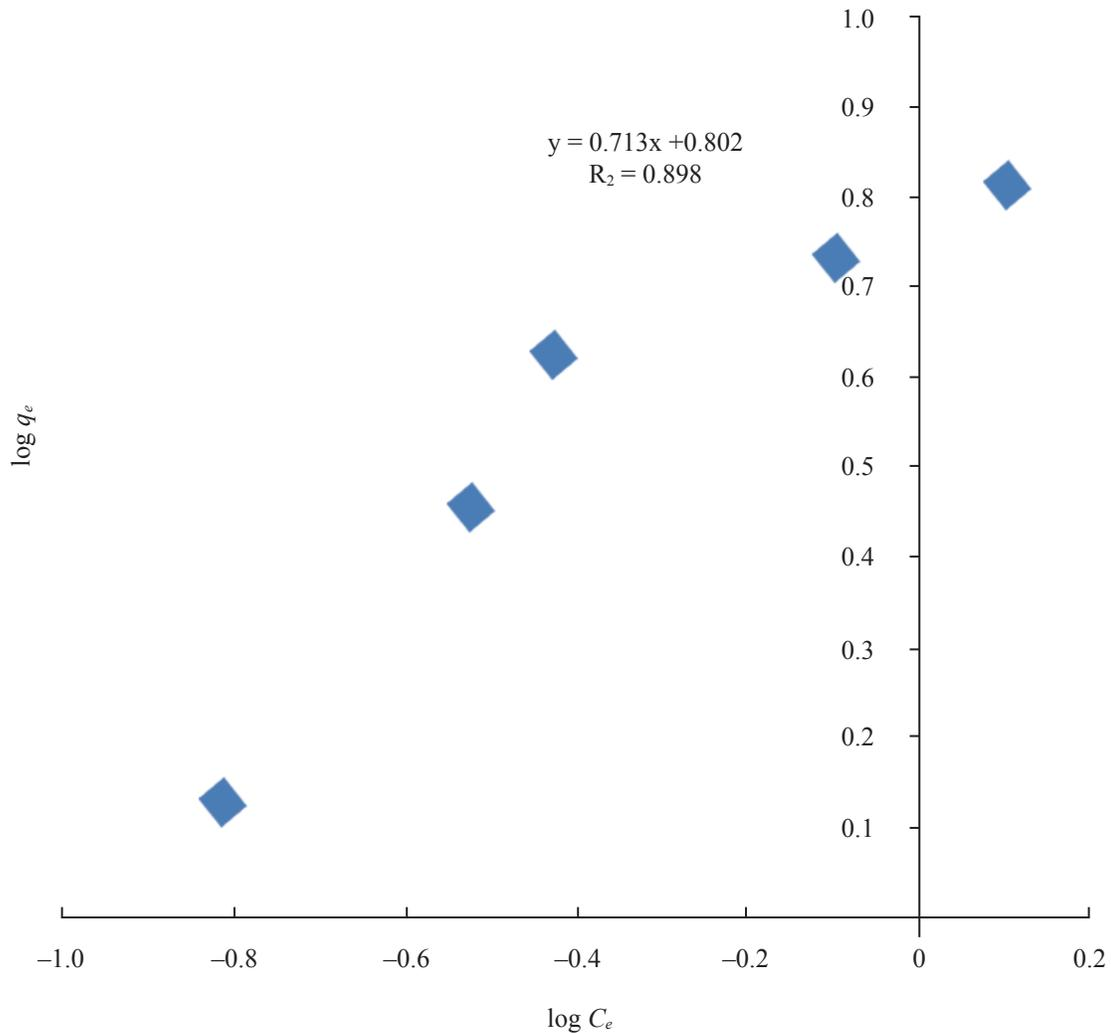
**Figure 6.** The graph of Freundlich isotherm for MB dye adsorption onto rambutan skin biosorbent.
