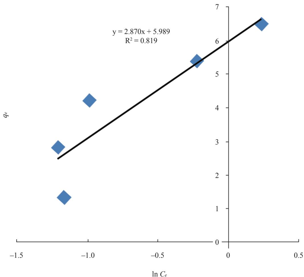
**Figure 7.** The graph of Temkin isotherm for MB dye adsorption onto rambutan skin biosorbent.
