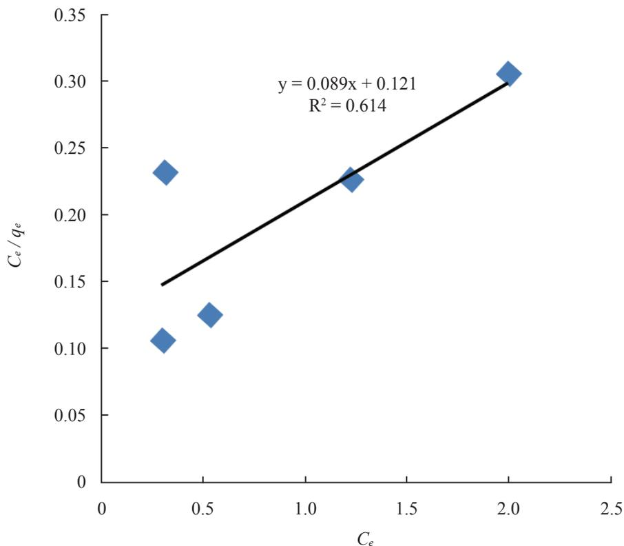
**Figure 5.** The graph of Langmuir isotherm for MB dye adsorption onto rambutan skin biosorbent.
