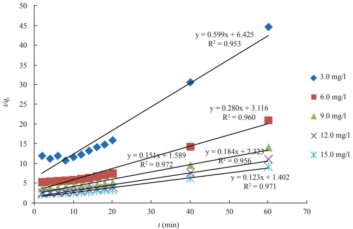
Figure 9. The pseudo-second-order kinetic model for MB dye adsorption onto rambutan skin biosorbent.
