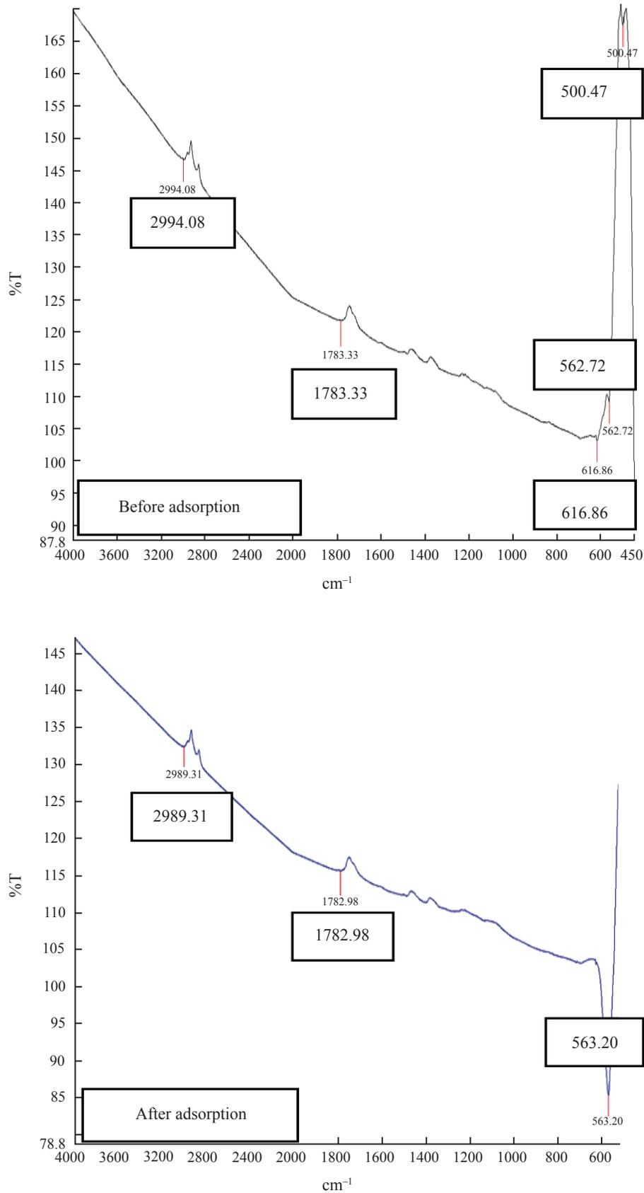
**Figure 1.** The FTIR Spectra of the rambutan skin before and after the adsorption process.
