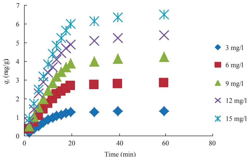
**Figure 2.** The effect of initial dye concentration on the adsorption capacity of the rambutan skin biosorbent.
